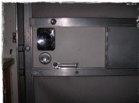
The first picture shows the screen being held with a strap. The strap is replaced often because the button fails. It also shows a sliding latch used to hold the screen door closed when the main door is open.
