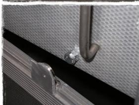
To solve the problem I used rare earth magnets and a fabricated angle bracket.
