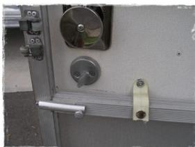
Anyone with a late '60's trailer is familiar with the strap button used to hold the screen door to the main trailer door.
