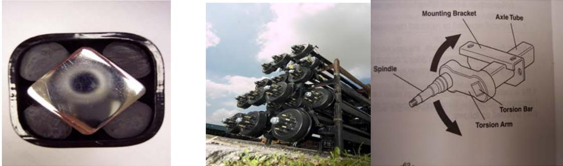
Airstream uses a unique independent suspension system that is contained within the axle. The simple compact design gives unparalleled performance compared with other suspension systems.
