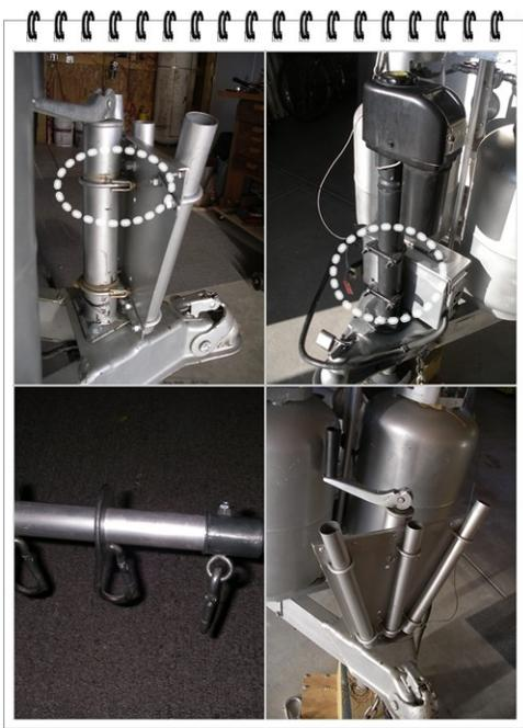
The pipes are electrical conduit with an ID (1 ¼) that will hold the poles. They are held to the plate (3/32 aluminum) with U bolts. The top of the plate is stiffened with ½ aluminum angle that has a rounded notch where it intersects the jack shaft. The plate is cut (on table saw) and the pipes mounted so that the outer pipes are 20 degrees off vertical. This assembly is held to the jack with muffler clamps.
